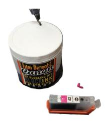
1. Replace orange plastic piece to bottom of cartridge. Fill syringe.
